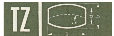
Barrel (TZ) and with Round Corners (TZR) Shape - One Side Curved Bezel - Sternkreuz TZ & TZR
